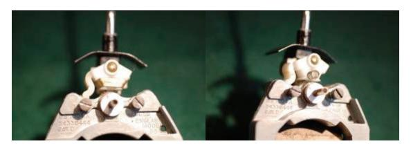
As you carefully remove the contact plate you will see a part that has two springs on both ends, and, a U-shaped contact with a spring under it. The white nylon piece is the turn detent device (action spring).
