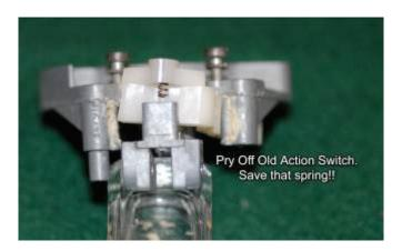
Carefully pry off the old broken action spring (above). With a Q-tip and solvent, clean off any old grease on the casting. Apply a couple of drops of clear machine oil in the moving part. We're now ready for re-assembly.
