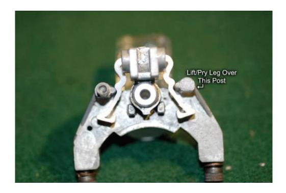
Lastly, pry the other arm up and over into position. (Now you can see why I avoided the taller post on the left!) You can try a different procedure, but this is the only one I found that works. With a small artist brush, apply white lithium grease in the areas where the detent works against the casting. Put plenty of grease in there and work the mechanism back and forth, but don't get too sloppy with the stuff.
