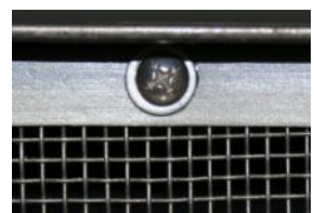
Early woven wire scuttle vent screen (above) - late expanded metal screen (below).
