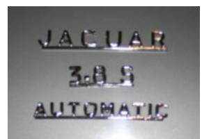
'Automatic' emblem on the trunk lid of early cars - not late cars
